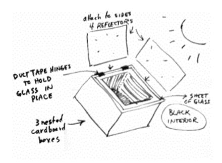
Above you have a solar oven design made with cardboard boxes, aluminum foil and a piece of window glass. Interior of the box is flat black paint.
